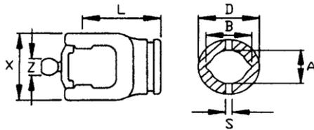
**CV Wide Angle 80° Inboard Yoke for Outer Tube**
