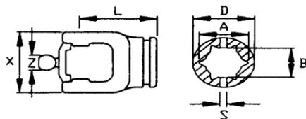
**CV Wide Angle 80° Yoke for Outer Tube**
